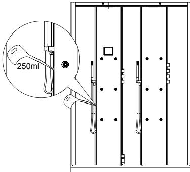
For decalcification, pour in 250ml of the liquid decalcifier (i. e. HOESCH special softening agent Art.Nr. 692101) and activate the process by keeping button 5 pressed for 10 seconds.
