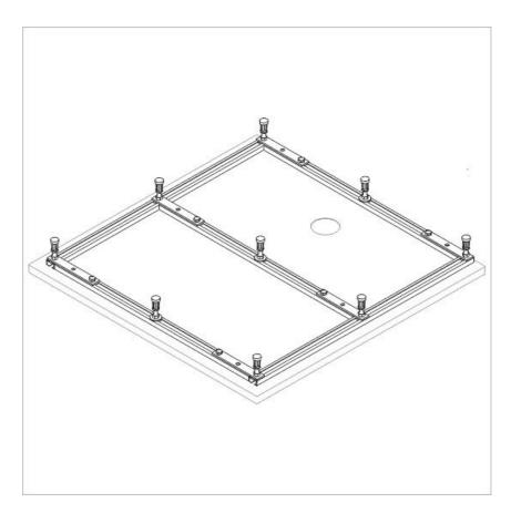
The base frame is a very easy, fast and stable shower tray installation system. The feet of the Hoesch frames can be adjusted in height.
