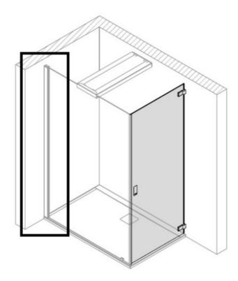
with stainless steel look for attachment of the glass panel (8 mm, glass provided by customer). The wall connection profile can be shortened to the desired length during fitting. Adjustment range of the wall connection profile: +/-8mm
