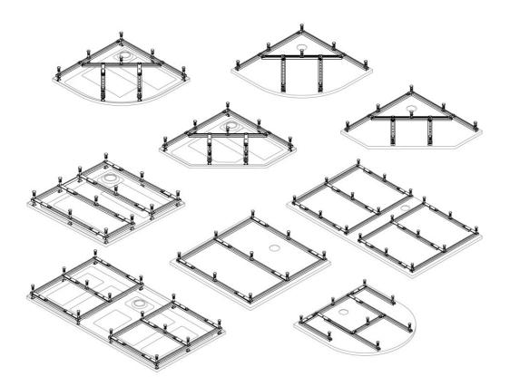
The base frame is a very easy, fast and stable shower tray installation system. The feet of the Hoesch frames can be adjusted in height.
