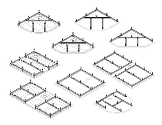
The base frame is a very easy, fast and stable shower tray installation system. The feet of the Hoesch frames can be adjusted in height.
