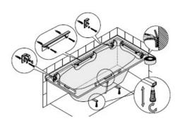
Mounting set for bathtubs consists of: 1 Pair of tub feet, 1 Set bathtub anchor, 1 Set tub strips, Wall connection profile
